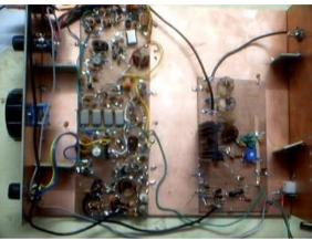
BITX single-band (20M) low cost, QRP SSB radio created in 2003 by Ashhar Farhan VU2ESE
